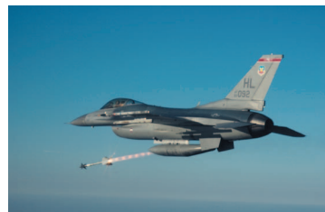
UPI Photo/Michael Ammons/Air Force/Landov LLC Heat-seeking missiles such as "Stinger" and "Sidewinder" use infrared sensors to measure gradients.
